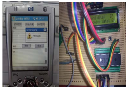
Fig.9 Characters to send and receive test pattern of MCU and mobile phone
