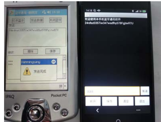
Fig.8 Characters to send and receive test pattern of PC and mobile phone
