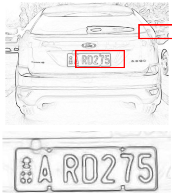
Fig5 Approximate localization results(above) and result of accurate localization(below)
