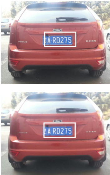
Fig3 Original image(above) and results of median filter(below)
