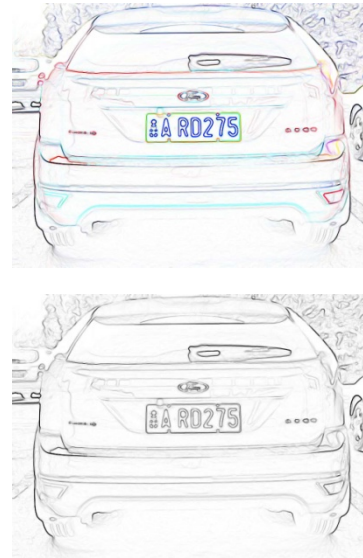
Fig4 Result of edge detection(above) and results of binarisation(below)
