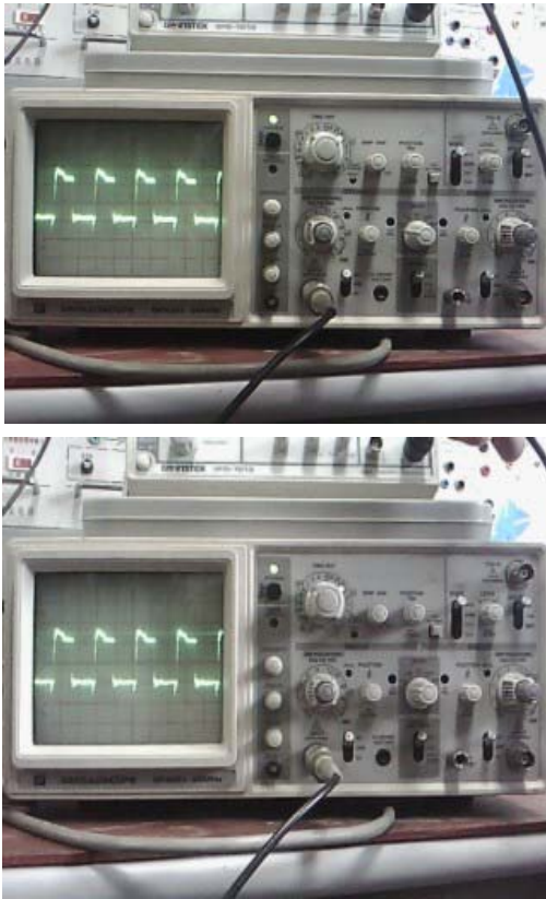
Fig. 6. Circuit SG3525 pin 11 and 14 pin waveform
