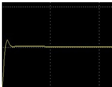
Fig.11 The step response of pitch channel
